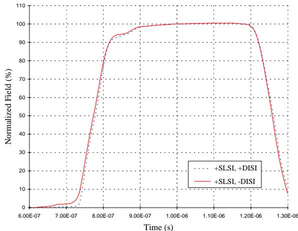
**Figure 2. Magnet field at 80kV PFN with MS and DS SLSI, in a 31.5 $\Omega$  kicker terminated with a short circuit, with and without a 12cm<sup>2</sup> DISI.**
