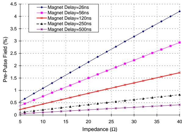
**Figure 4 Calculated pre-pulse field amplitude as a function of magnet impedance and delay time without ferrites.**
