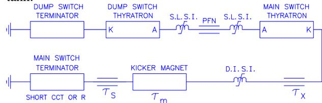
Figure 1. Block diagram of pulse generator and kicker magnet test system.
