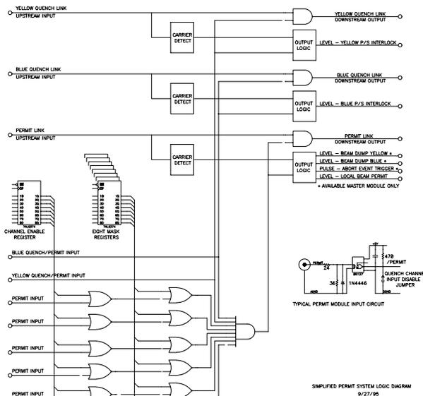
Figure 2: Beam and quench protection permit links logic diagram.
