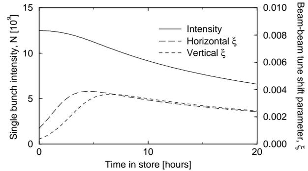
Figure 6: Long range tune shift evolution, per IR.
