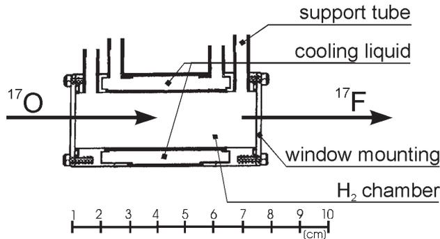
Fig. 2. A simplified cross-section of the cylindrical gas target used. The diameter of the windows is 1.27cm
