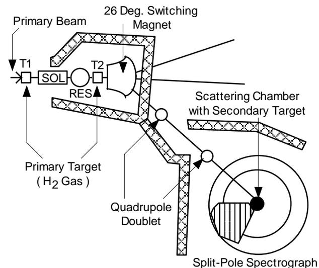
Fig. 1. Floor plan of the ATLAS radioactive beam region. The future (T1) and present (T2) positions of the primary gas target are shown as are the beam transport elements to the secondary target at the spectrograph. The relative positions of the super-conducting solenoid (SOL) and resonator (RES) which will be installed are also indicated.
