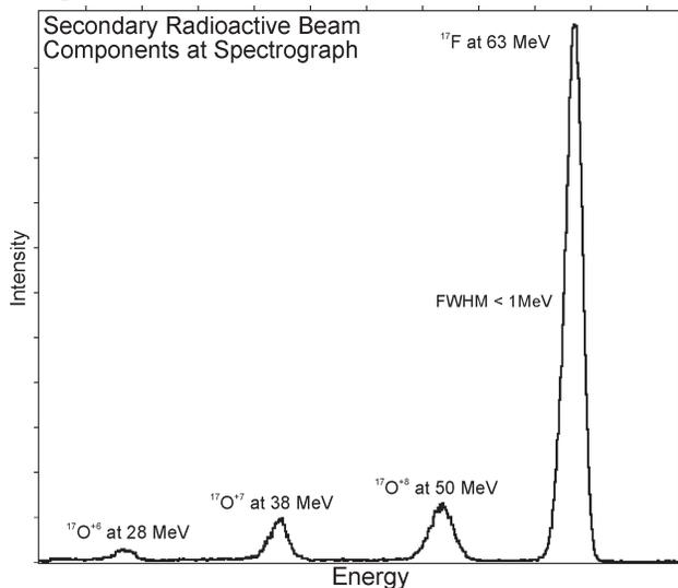
Fig. 4. The energy spectrum of the secondary beam in the ATLAS spectrograph at  $0^\circ$ .
