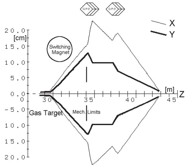
Fig. 3. The calculated envelope of the produced  $^{17}\text{F}$  beam from the production target, located at 30m, to the reaction target, located at 43m. The quadrupole doublets are in a YX-YX-configuration.
