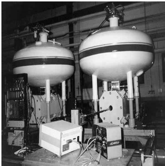
Fig. 4 Solenoids under test at MIT-Bates. Dec. 1996.
