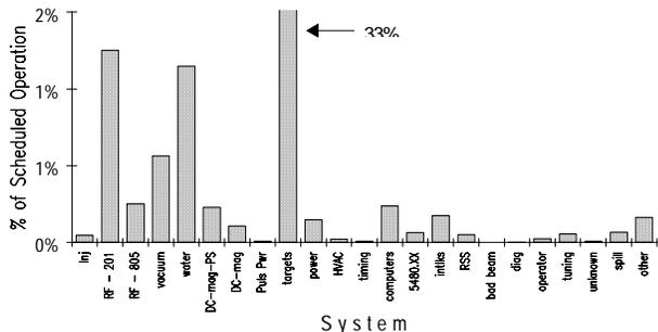
Figure 1: Causes of downtime for H<sup>+</sup> beam delivery to Area A histogrammed by system.
