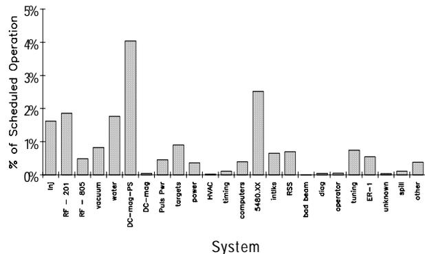
Figure 3: Causes of downtime for H<sup>+</sup> beam delivery to the Lujan area histogrammed by system.
