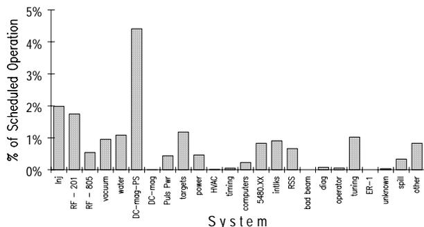
Figure 2: Causes of downtime for H<sup>+</sup> beam delivery to the WNR area histogrammed by system.
