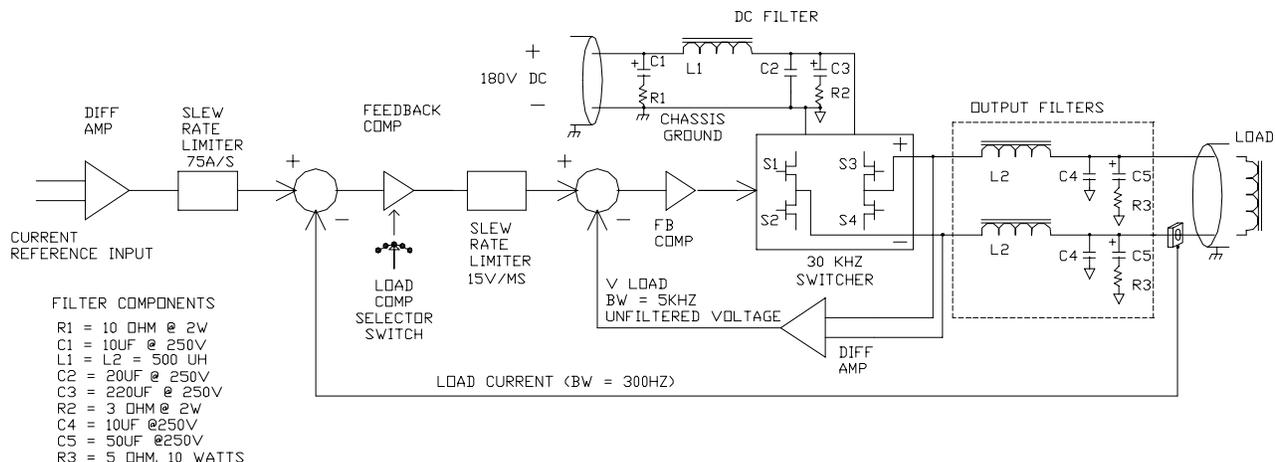
Figure 1, Regulator Configuration
