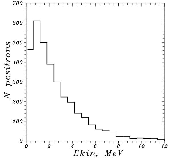
Figure 2: Kinetic energy distribution for positrons emitted from tungsten target  $0.3 \times 10 \times 10$  mm under impact of SR photons from HERA-e  $8T$  wiggler.
