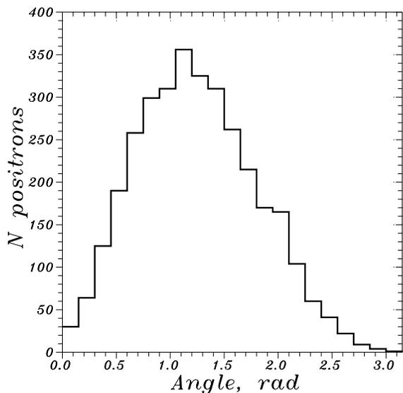
Figure 3: Distribution over  $\Theta$  for positrons from 1-20 MeV SR photons, tungsten target size  $0.3 \times 10 \times 10$  mm, all positrons are emitted from target.
