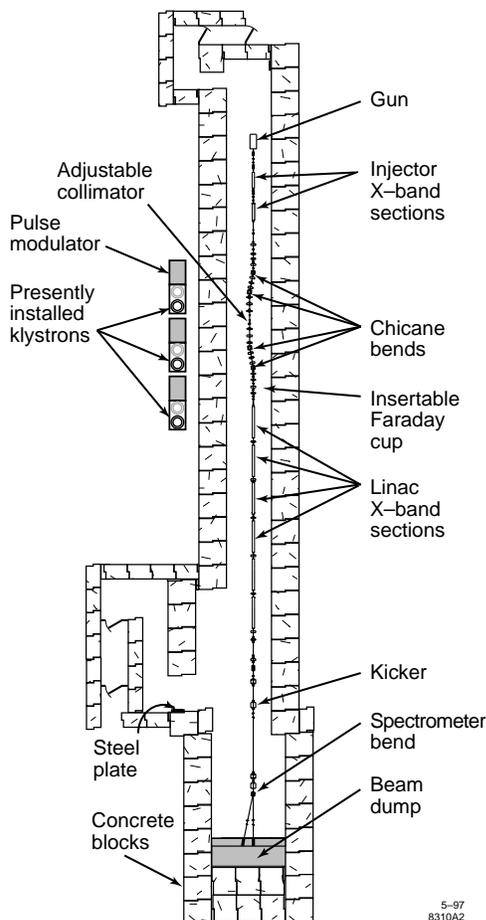
Fig. 1. Plan view of the NLC Test Accelerator. The length of the beam line from gun to dump is 43 m.
