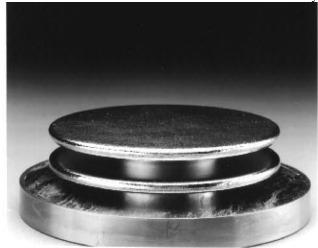
Figure 3: Niobium bellows tuner assembly. The tuner can be pressurized with helium gas and provides a two millimeter range of motion with 0 - 1 atmosphere internal pressure. A 70 kHz tuning range results.
