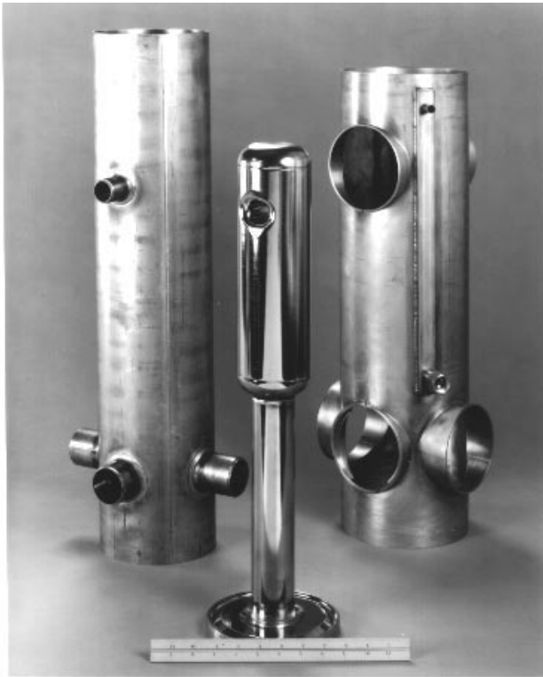
Figure 2: Major components of the niobium quarter-wave coaxial-line cavity prior to final weldment. Elements shown are the quarter-wave line and drift-tube, the 6.5 inch OD niobium outer housing and the 7.5 inch OD stainless-steel outer jacket
