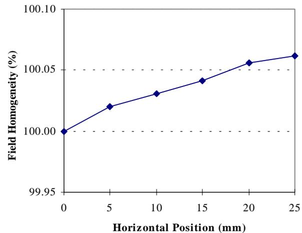
Fig: 3 Homogeneity of integrated field through the cylindrical magnet design as a function of horizontal position.
