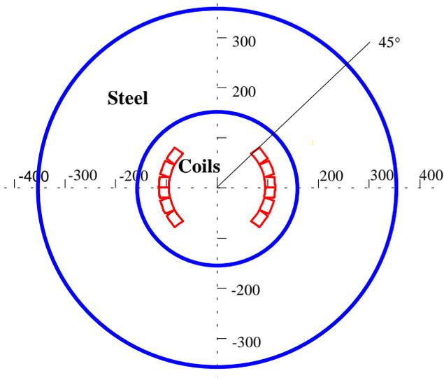
Fig: 1 Cross section through cylindrical design magnet showing coil and iron radial distribution.
