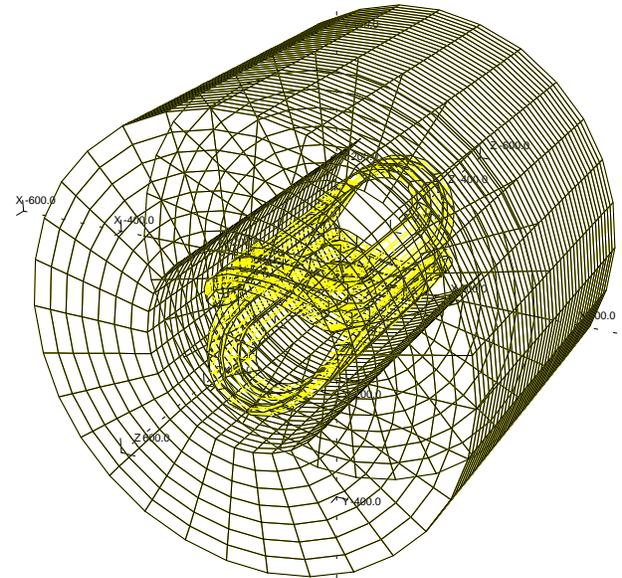
Fig: 2 Orthographic projection showing cylindrical magnet coil and iron geometry.
