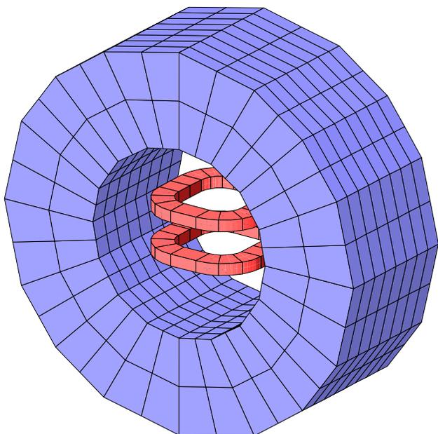
Fig: 4 Orthographic projection showing Helmholtz configuration magnet in three dimensions.
