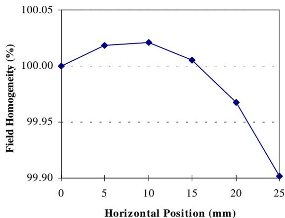
Fig: 5 Homogeneity of integrated field through the Helmholtz configuration magnet as a function of horizontal position.
