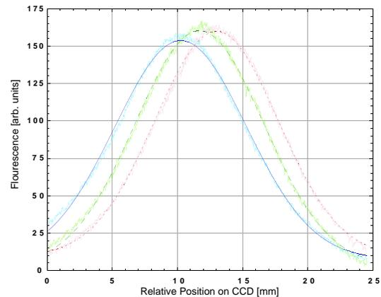
Figure 3: Horizontal beam profiles measured for different longitudinal velocities of a particular beam. The lines are gaussian fits to the data. The solid line is  $\Delta v = -279.6\text{m/s}$ , the long-dashed line is  $\Delta v = 0$ , and the short-dashed line is  $\Delta v = 279.6\text{m/s}$ . For clarity the three curves have been renormalized to the same height.
