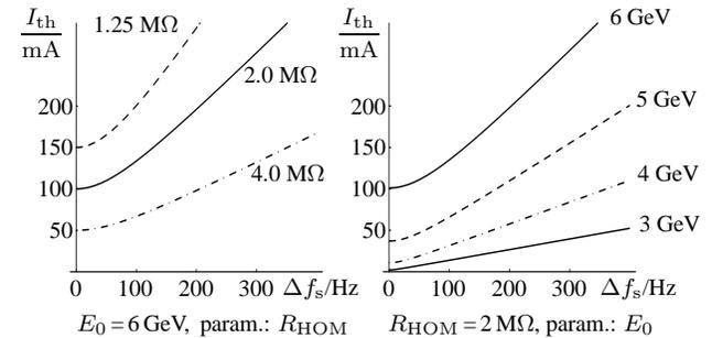
Figure 3:  $I_{th}(\Delta\omega_s)$  from eq. (8),  $f_{HOM} = 500 \text{ MHz}$ .
