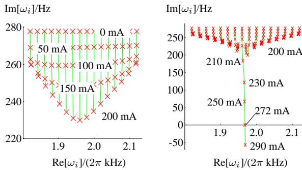
Figure 2: Evolution of the  $\omega_i$  with  $I_b$ .
