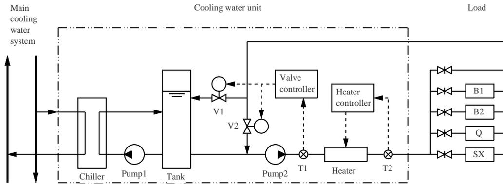
Fig. 2 Block diagram of the prototype cooling water unit.
