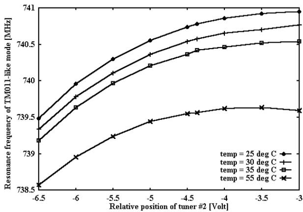
Figure 1: Resonance frequency of the  $TM_{011}$ -like mode of the DORIS-I cavity as a function of the second tuner position (measured in unit of volt) as well as the cavity cooling water temperature. The first tuner was properly repositioned such that the resonance frequency of the cavity fundamental mode was kept to be of 499.666 MHz, which was the accelerating frequency of the SRRC storage ring.
