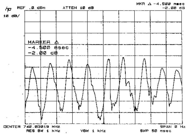
Figure 6: Quasi-periodical variation of the oscillation amplitude of the synchrotron upper dipole mode of  $n = 97$  (742.03019 MHz) as a function of time.
