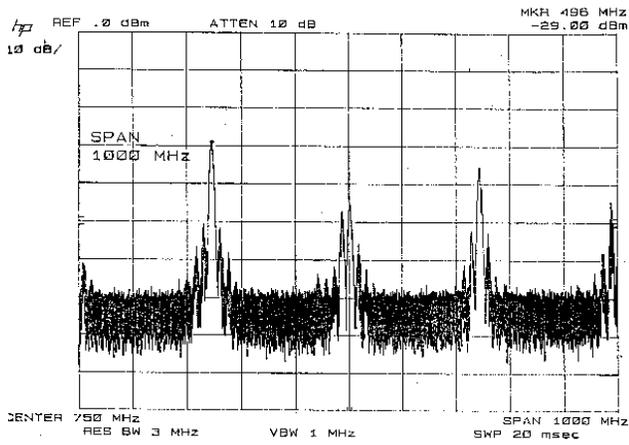
Figure 4: Beam spectrum when the second tuner of the cavity RF#1 was located close to the on-resonance position (tuner #2 position is 5.3 Volt).
