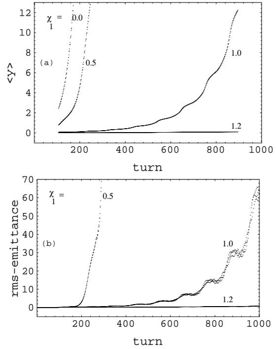
Figure 1: Multi-particle simulation results showing stabilization of the SHT motions of (a) the centroid, and (b) the rms-emittance of a Gaussian beam by  $\chi_1$ , where the standard SHT stability limit is  $\Upsilon_{SHT} = 1$  (when  $\chi_1 = 0$ ). In these figures,  $\chi_0 = 0$ ,  $\Upsilon = 1.65$ . According to Eq. (11), when  $\chi_1 = 1.2$ ,  $\Upsilon_{SHT} = 1.73$ .
