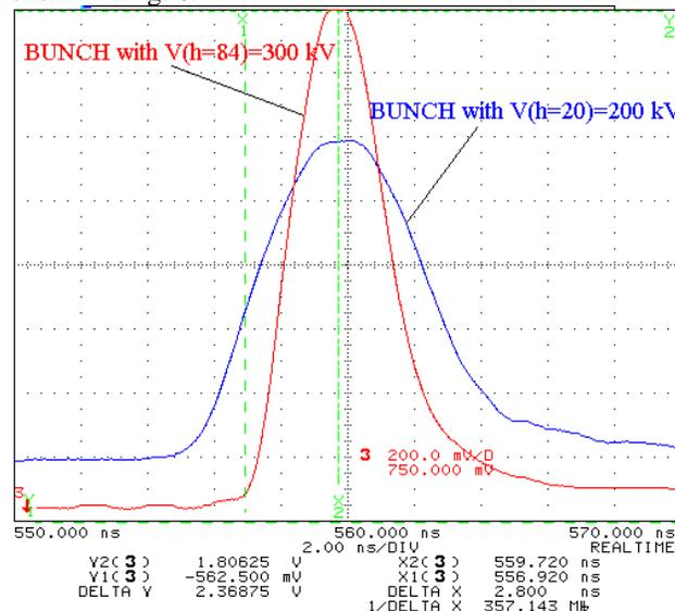
Figure 6: Single bunch rotation: bunch length  $\approx 5$  ns
