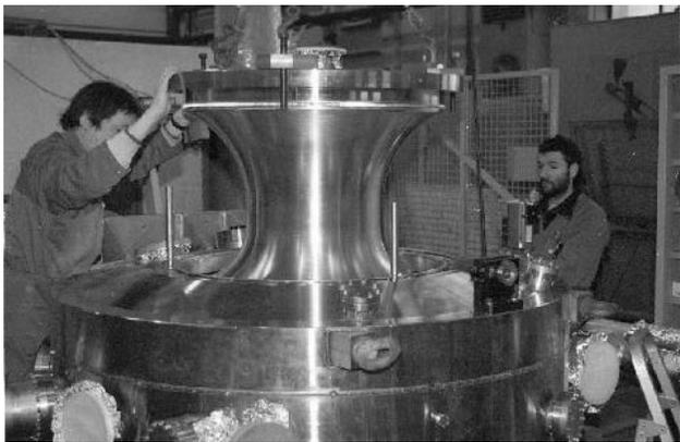
Figure 1: Mounting the center electrode into the cavity.
