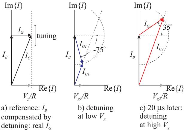
Figure 2: Varying tuning angle with non-adiabatic variation of the gap voltage.
