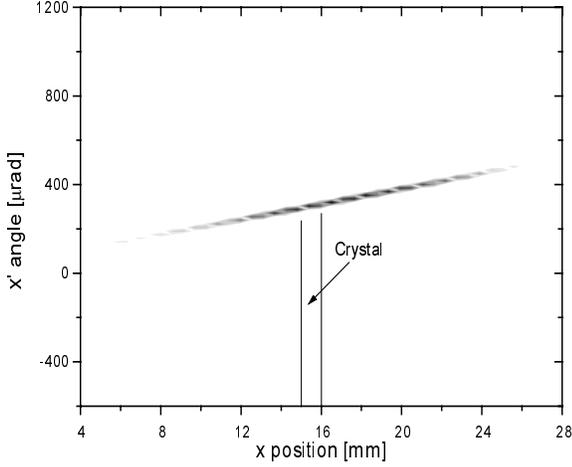
Figure 2: Horizontal phase space of the 450 GeV/c protons incident on the germanium crystal. This measurement stems from two drift chambers located 36.9 and 0.5 m upstream of the crystal (see Fig. 4). The horizontal width of the bent crystal is indicated to illustrate the relevant phase space for this experiment.
