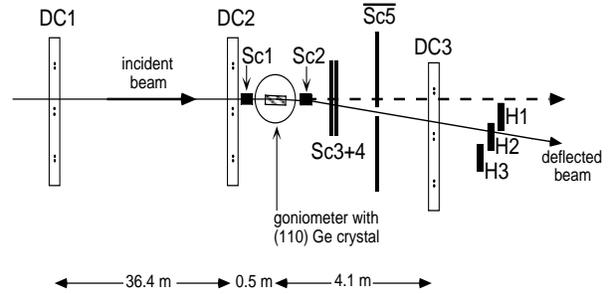
Figure 4: Schematic view of the experimental arrangement. Protons are deflected horizontally by the bent germanium crystal. Scintillators Sc1-4 are trigger counters for incident beam particles, H1, H2 and H3 for deflected particles. SC5 is a veto counter used during crystal alignment. Driftchambers DC1, DC2 and DC3 define the incoming and exiting beams, respectively.
