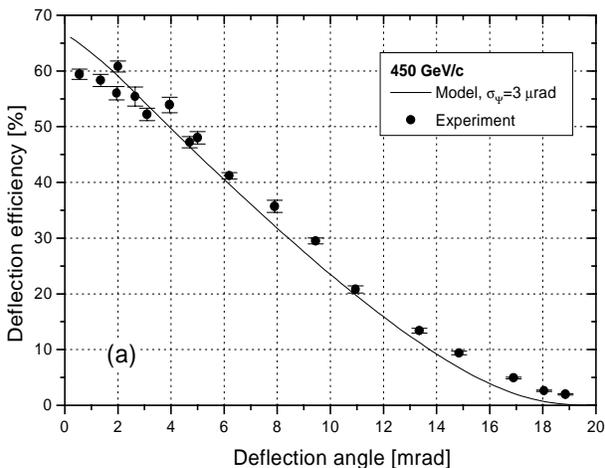
Figure 5: Deflection efficiencies measured for  $450 \text{ GeV}/c$  protons incident on a bent germanium crystal (dots) compared to calculations following the model of [6]. For details, see text.
