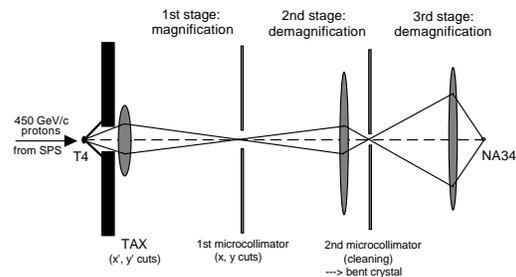
Figure 1: Conceptual layout of the H8 micro-beam (horizontal projection). For the present experiment, the cleaning collimator was removed, the bent crystal installed at its place and the beam tuned to be parallel to the crystal. For details, see text.
