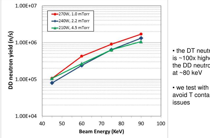
• the DT neutron yield is ~100x higher than the DD neutron yield
