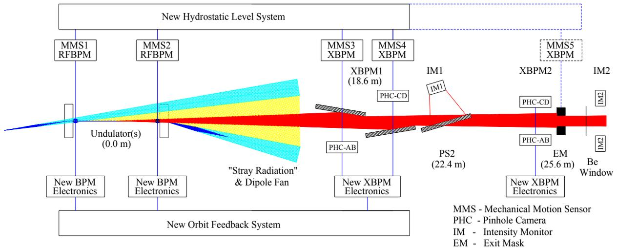
Figure 5: In the APS-U orbit feedback system, the XBPM system is responsible for measuring the x-ray beam angle and monitoring the x-ray beam intensity and position outside of the feedback loop.
