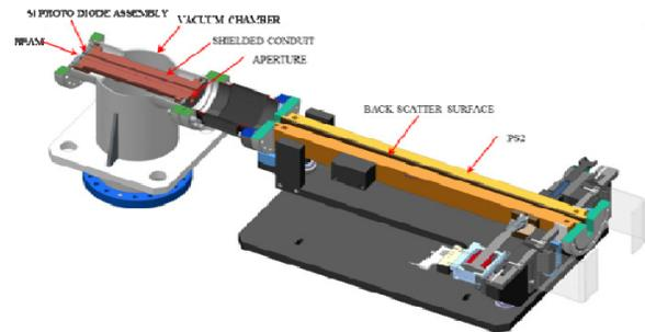
Figure 4: IM1 uses Cu K-edge XRF to measure the x-ray beam intensity when the photon shutter is closed.
