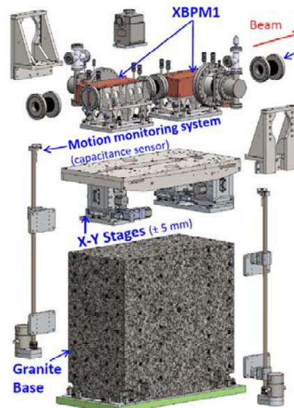
Figure 1: The GRID-XBPM for the APS-U high-heat-load front end.
