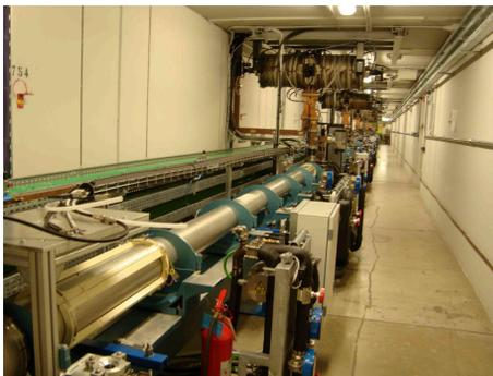
Figure 2: One of the SLED equipped BTW structures.
