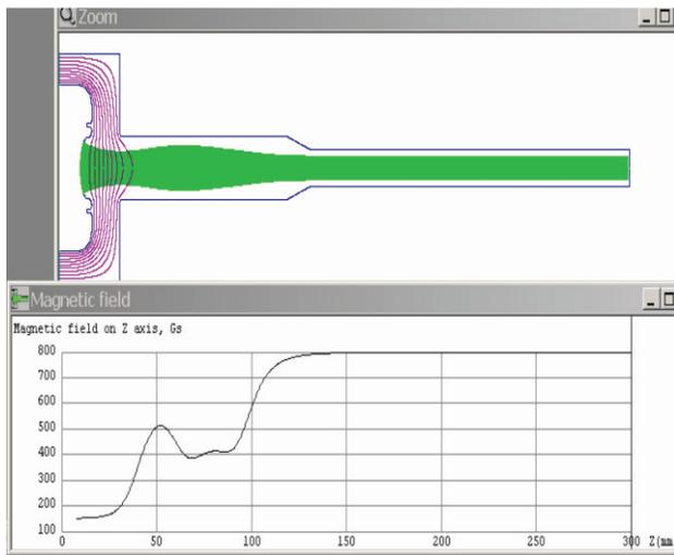
Figure 4: an example of electron beam matching in PX MBK. Horizontal divisions are 50 mm, and vertical divisions are 100 G.
