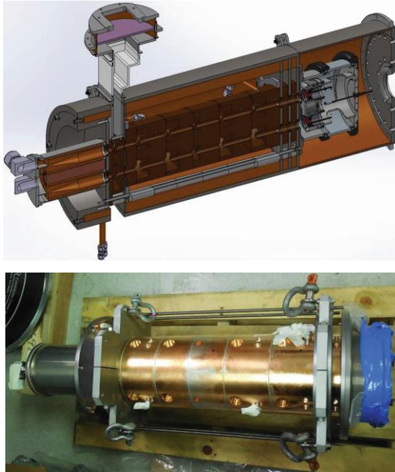
Figure 2: The 6-beamlet quadrant is to produce 2.5 MW at a 10 Hz repetition rate; the tube (at top) is shown inside the solenoid, and the cavity structure with the collector (at bottom) is photographed without the gun.
