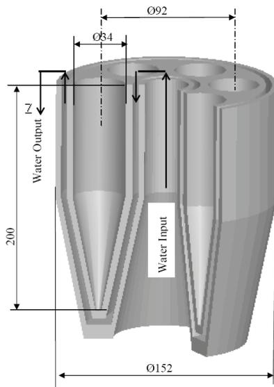
Figure 5: The collector with 6 cells for 6 beam-lets (see explanations in the text).
