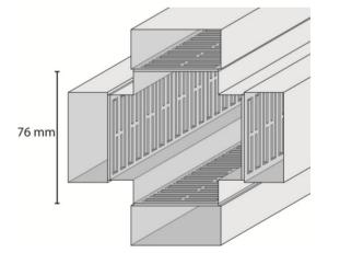
Figure 1: Metamaterial waveguide assembled from four WR187 waveguides (47.55 x 22.15 mm) with CSRRs machined into inner face of assembled structure.
