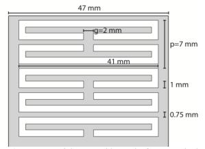
Figure 2: Metamaterial waveguide made from standard WR187 waveguide with CSRRs machined into one face of the guide.
