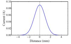
Figure 4: Test bunch current profile used in the wakefield simulations.
