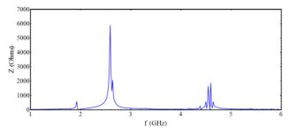
Figure 6: Longitudinal wake impedance shown as a function of frequency.
