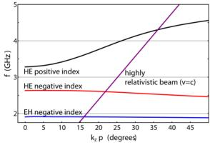
Figure 3: Dispersion curves of TM modes in the metamaterial waveguide. Two modes exist that couple to the electron beam, a negative refractive index mode at 2.5-2.6 GHz (red) and a positive index mode at 3.5-4.5 GHz (black). The relativistic electron beam dispersion line is also shown  $(2\pi f = k_z c, \text{ purple})$ .
