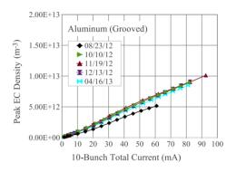
Figure 8: TE wave data from the grooved aluminum chamber in L3 also shows a step increase in EC density after the earliest measurement.
