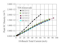
Figure 4: TE wave data with ten bunches from the grooved TiN-coated chamber at L3.
