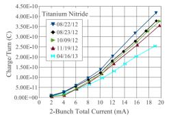
Figure 3: 2-bunch SPU data from the TiN-coated chamber at 15W (see Fig. 2) is integrated to obtain charge/turn. The data shows monotonic conditioning with beam dose. This includes the earliest conditioning with less than 0.5 amphours.
