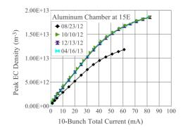
Figure 7: TE wave ten bunch data from the bare aluminum chamber at 15E shows a step increase of about 40 percent in EC density after the earliest measurement.
