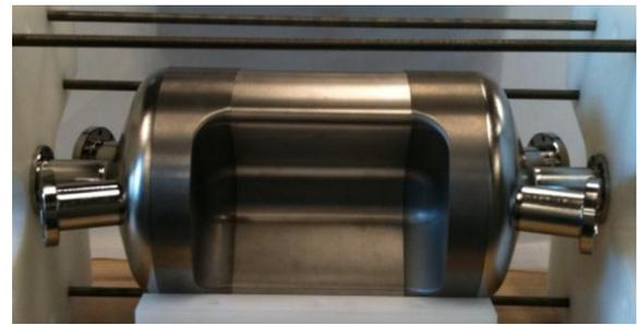
Figure 5: Clamped cavity for frequency measurement.
