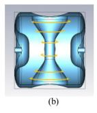
Figure 2: field line sketch of a spoke resonator (a) electric and (b) magnetic [1].
