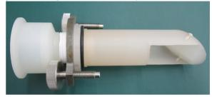
Figure 2: Single injection quill used for FRIB  $\beta$ =0.53 HWR cavity BCP processing.
