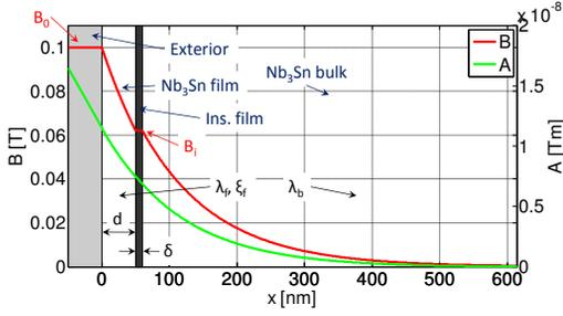
Figure 1: Geometry of the structure under consideration. The amplitudes of the magnetic field and the vector potential are plotted as a function of distance into the structure.
