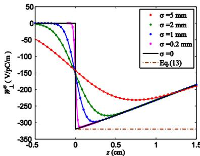
Figure 3: (dots) transverse ECHO wake potentials, and (solid) wakes reconstructed from  $W_{\perp,ECHO}^{2mm}$ .
