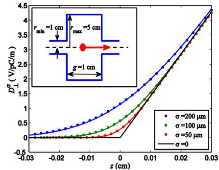
Figure 4: (inset) geometry; (dots) wakes calculated by ECHO and (solid) reconstructed from  $W_{\perp,ECHO}^{1mm}$ .
