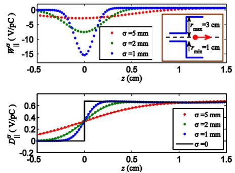
Figure 2: (inset) step-out geometry; (top) ECHO wake potentials; (bottom) same with singular parts subtracted (dots), and (solid) wakes reconstructed from  $W_{\parallel, ECHO}^{2mm}$ .
