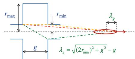
Figure 1:  $\lambda_g$  for a cavity with  $r_{\max}/r_{\min} \geq 2$  and  $g/r_{\min} \geq 2^{-1/2}$ .
