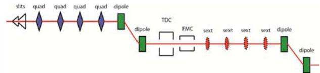
Figure 3: The schematic of a beamline for producing shaped electron bunches.
