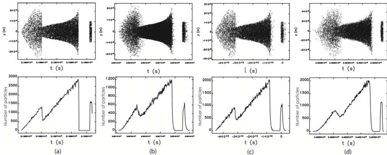
Figure 5: Distributions of the electrons (2D and integrated over y-axis) in the drive and witness bunches after the mask and the EEX as computed by Elegant: (a) in the first order of matrix elements, (b) in the third order of matrix elements, (c) in the first order with the second order matrix element  $T_{555}$  artificially included, and (d) in the third order with correcting sextupoles turned on.
