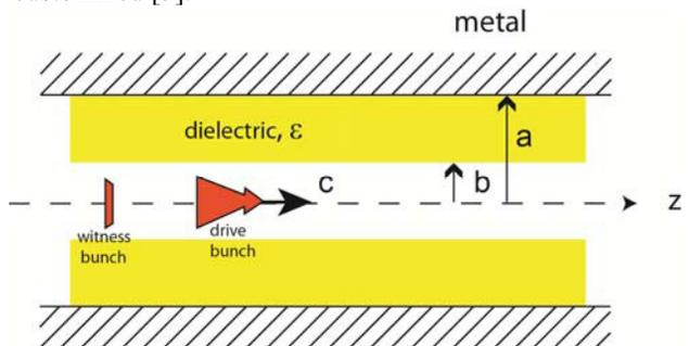
Figure 1: The schematic of a dielectric loaded waveguide with shaped electron beams traveling on axis.
