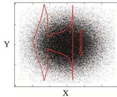
Figure 4: The shape of the mask plotted on top of the Gaussian bunch.
