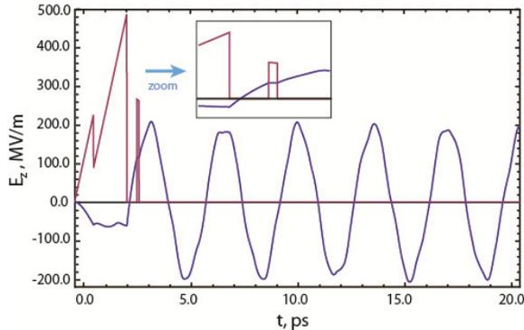
Figure 2: The current profiles of the drive and the witness bunches (red line) and the wakefield (blue line) excited by the pair of bunches in a proposed DWA configuration.
