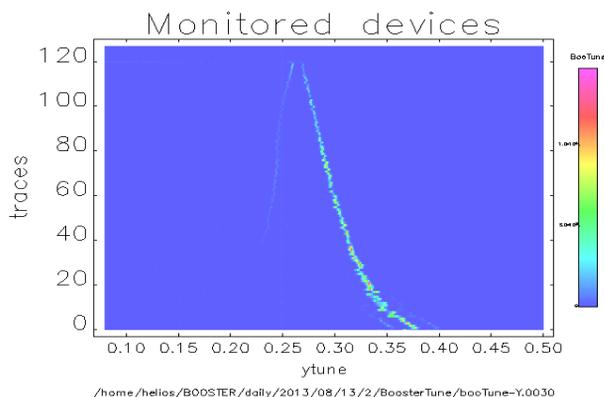
Figure 5: Tune plot of a fully coupled booster beam. The bright trace is the horizontal tune and the dim trace on the left is the vertical tune. Each trace represents 1.8 ms in time.
