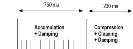
Figure 1: Accumulation of high-charge single-bunch beam in the PAR.
