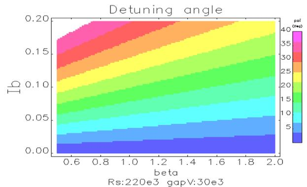
Figure 4: Detuning requirement as a function of beam current and coupling coefficient of the RF12 cavity.
