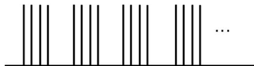
Figure 2: A multiple bunch train fill pattern.
