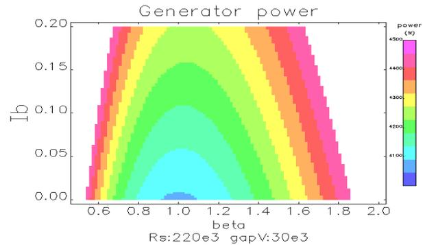
Figure 3: Power requirement as a function of beam current and coupling coefficient for RF12.
