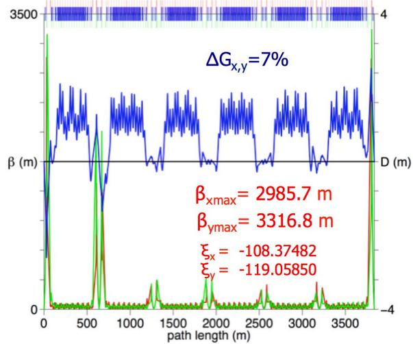
Figure 6: Betatron functions after the betatron wave is created through the IP 6.
