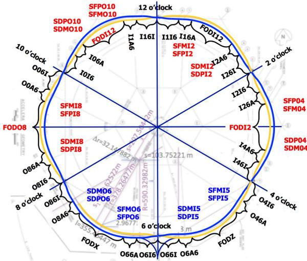
Figure 4: RHIC 24-sextupole circuits schematic.
