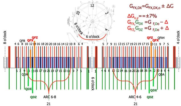
Figure 5: The quadrupole pairs to induce the beta wave are labeled QFX and QFZ, and QDX and QDZ at the beginning and end of the arcs.
