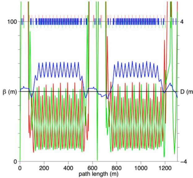
Figure 3: Details of the betatron functions around the IP for the  $\beta^*=75$  cm.
