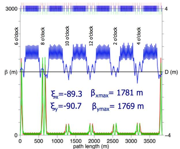
Figure 2: Betatron functions of the RHIC 90° degrees lattice with the  $\beta^*=80$  cm. Two interaction regions at 6 and 8 o'clock have the same beam size.
