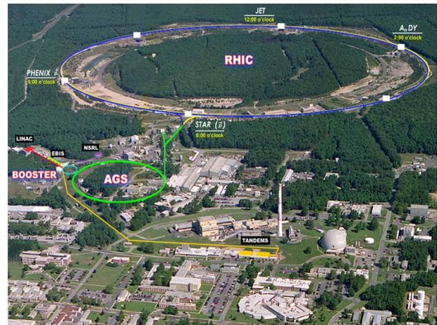
Figure 1: The RHIC accelerator complex shows the major components Linac, Booster, Alternating Gradient Synchrotron (AGS), and RHIC. The Electron Beam Ion Source EBIS is an additional important element.
