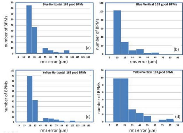
Figure 2: Resolution of turn-by-turn BPM measurements in histogram format for the blue/yellow ring horizontal plane (a)/(c) and vertical planes (b)/(d).
