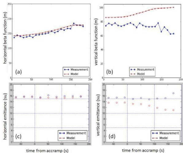
Figure 3: Model (red) and measured (blue) beta functions in the horizontal/vertical planes at 255 GeV during the final beta squeeze (a/b); IPM emittances (95%, normalized in mm-mrad) reported using the model (red) and measured (blue) beta functions in same planes (c/d).
