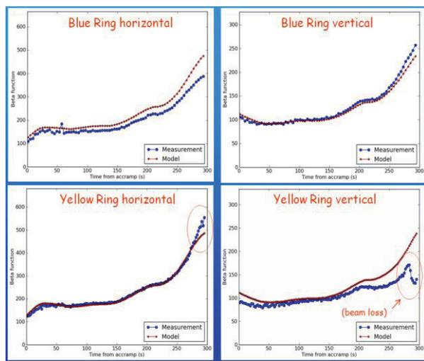
Figure 4: Model and measured beta functions at the 4 RHIC IPMs during acceleration of protons to 255 GeV.
