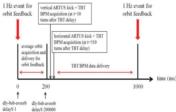
Figure 1: Conceptual sketch of carefully orchestrated timing to allow for turn-by-turn BPM acquisitions interleaved with BPM acquisitions required by orbit feedback during beam acceleration.
