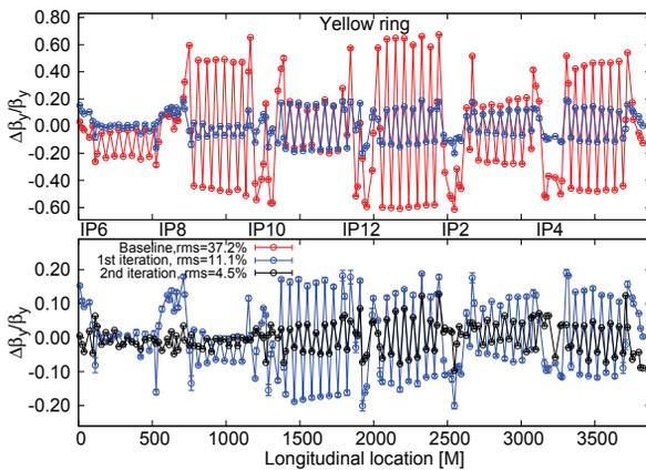
Figure 6: Baseline and corrected vertical beta-beat with error bars for the Yellow ring. The peak beta-beat was reduced from 60% to 20% after the first iteration of correction, and further reduced to 10% after the second iteration.
