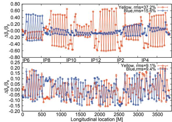
Figure 1: Measured beta-beat with error bars in the horizontal (bottom) and vertical (top) plane for both rings at RHIC. 15% peak beta-beat was observed in the horizontal plane for both rings. A 30% vertical peak beta-beat was found in the Blue ring and 60% in the Yellow ring
