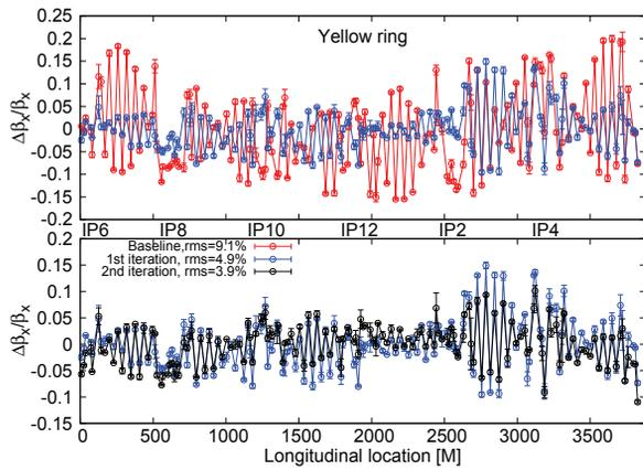
Figure 5: Baseline and corrected horizontal beta-beat with error bars for the Yellow ring. The peak beta-beat was reduced from 15% to 12% after the first iteration of correction, and further reduced to 10% after the second iteration.
