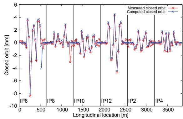
Figure 7: Measured and computed horizontal closed orbit for correction of arc beta-beat in the Yellow ring.
