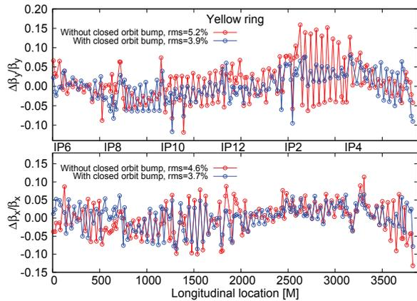
Figure 8: Horizontal (bottom) and vertical (top) residual beta-beat with and without the horizontal closed orbit bump displayed in Fig. 7 for the Yellow ring. Peak beta-beat was reduced to 7% for both planes with the closed orbit bump.
