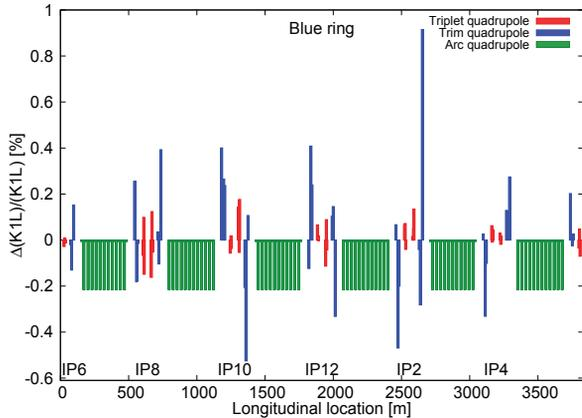
Figure 2: Relative changes of quadrupole integrated strength as a function of quadrupole locations in the Blue ring.
