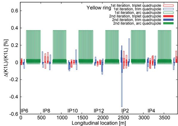
Figure 4: Relative changes of quadrupole integrated strength as a function of quadrupole locations in the Yellow ring for the first iteration (hollow bars) and second iteration (solid bars), respectively.
