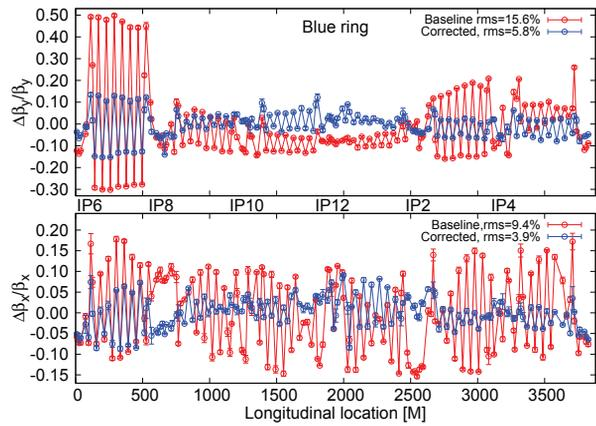
Figure 3: Baseline and corrected horizontal (bottom) and vertical (top) beta-beat with error bars for the Blue ring. Horizontal peak beta-beat was corrected from 15% to 8%, while vertical peak beta-beat from 40% to 14%.
