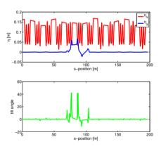
Figure 4: New fs-slicing optics that provides the spatial separation of the energy sliced beam in the new upgrade lattices.
