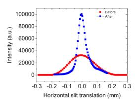
Figure 6: Comparison of the horizontal beam profile before and after the upgrade measured at one user beamline showing the factor of three improvement in brightness.
