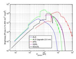
Figure 1: Comparison of the ALS brightness before and a after the low emittance upgrade with several other existing light sources.
