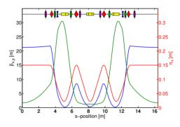
Figure 2: ALS upgrade lattice with 2.0 nm natural emittance at 1.9 GeV.
