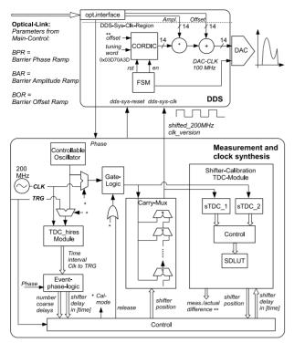
Figure 3: The block diagram of the system. The additional path for the combined mode is marked with (\*\*).
