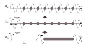
Figure 1: The procedure for beam pre-compression with the Barrier Bucket method (simplified).
