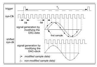
Figure 2: Principle of the phase accurate waveform generation by modifying the DAC data or, alternative, the DAC clock.
