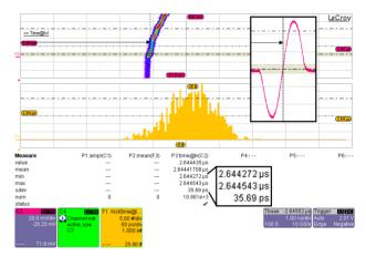
Figure 4: Jitter measurement between the trigger signal and the generated sine wave.
