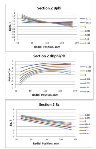
Figure 2:  $B_{\phi} dB_{\phi}/dr$ , and B ys. r for section 2. The different colors represent different ellipse asymmetries.
