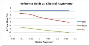
Figure 3:  $B_{\phi}$ , and  $-B_{\phi}$  in Tesla and  $dB_{\phi}/dr$  in T/m on the reference orbit for different ellipse asymmetries.
