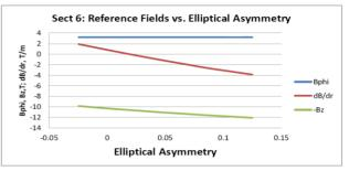
Figure 6:  $B_{\phi}$ ,  $dB_{\phi}/dr$ , and  $-B_z$  on the reference orbit as a function of elliptical asymmetry.
