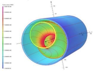
Figure 1: 3D layout of coils for the HCC channel. Note that the HS coils are placed in an external solenoid field.
