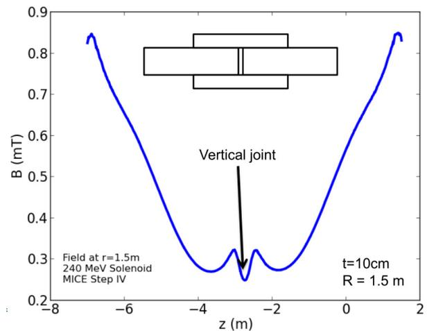
Figure 6: Modulus of the residual stray field at a radius of 1.5 m (beam height) for 200 MeV flip mode. The vertical gap is doubled up using two backing plates, each 40 cm long.
