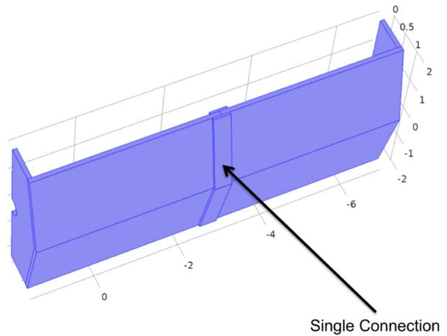
Figure 5: Concept of doubling up a vertical gap.
