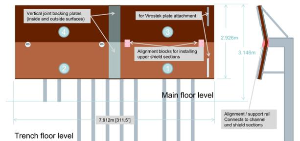
Figure 2: MICE partial return yoke.
