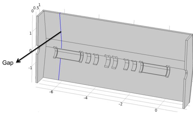
Figure 3: Geometry: Vertical gap in shield.
