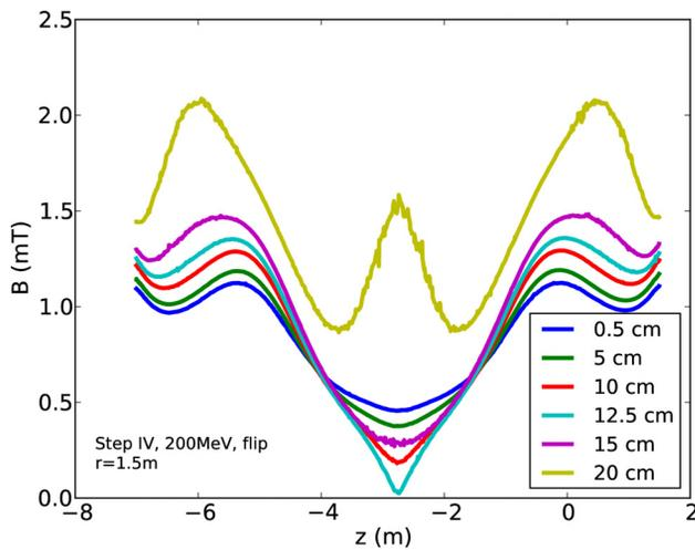
Figure 7: Modulus of the residual magnetic field at a radius of 1.5 m. The simulation assumes a horizontal gap in the PRY at beam height.
