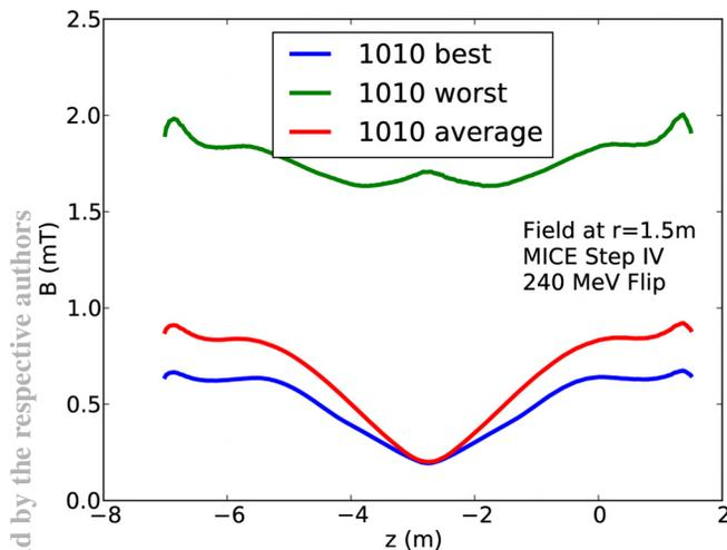
Figure 8: Stray magnetic field for different 1010 steels at a radius of 1.5 m (PRY finishes at a radius of about 1.35 m) and vertically at beam height.
