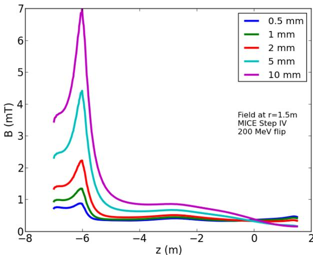
Figure 4: Modulus of the magnetic flux density at a radius of 1.5 m for 200 MeV flip mode assuming a vertical gap at  $z = -6$  m.
