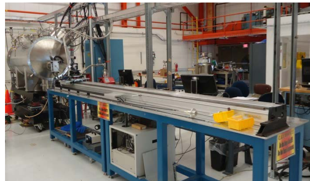
Figure 1: SCU horizontal magnetic measurement system with 3.5-m linear stage for Hall probe scans. SCU0 cryomodule is on the left.
