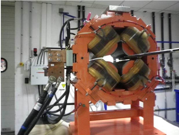
Figure 3: Hall probe median plane measurement.
