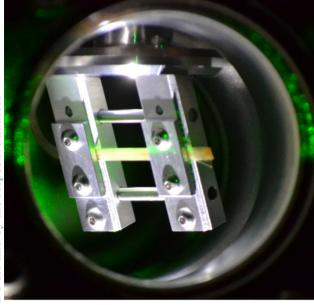
Figure 4: Fiber holder assembly in situ.
