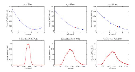
Figure 6: Top Row –Beam widths measured with YAG screens along the beamline (blue). Beam width measured with FMD plotted at the measured z- distance (red). Bottom Row – The averaged beam profile as measured with FMD.
