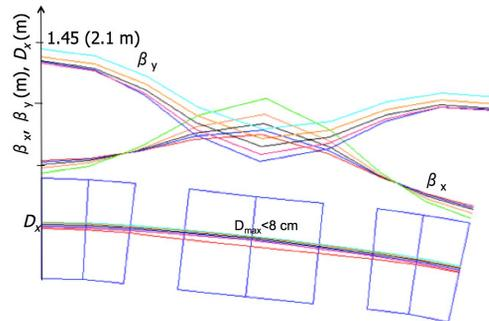
Figure 1: Betatron and dispersion functions in a gantry cell for the treatment energies.
