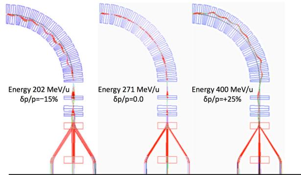
Figure 9: The 90°-superconducting gantry shown with carbon ions passing with three energies 202, 271, and 400 MeV/u under the fixed magnetic field, with scanning magnets. Positions of  $\pm 10$  cm at the patient are magnified.
