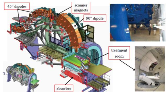
Figure 5: The whole structure of the Heidelberg carbon gantry with detail of the treatment room on the right side.
