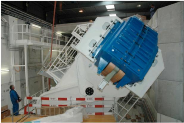
Figure 2: The proton top-notch proton therapy facility at PSI, with the large bending magnet at the end.
