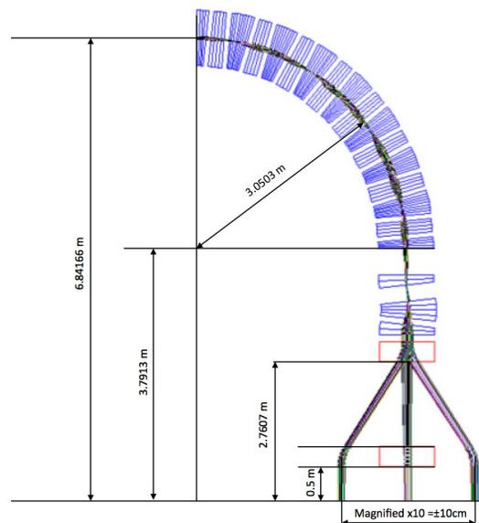
Figure 10: The layout of the 90° superconducting fixed field carbon gantry designed to fit to the CNAO eccentric gantry.
