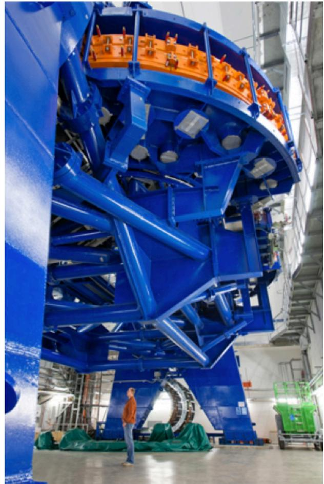
Figure 4: The Heidelberg gantry with a visitor. The large 45° magnet is shown above.
