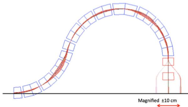
Figure 3: Our proton gantry design eliminates need for the large dipole and provides always 90° angle to the skin.
