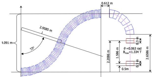
Figure 7: The carbon ion superconducting fixed field isocentric gantry layout. The scanning magnets are 30 cm long with a maximum required magnetic field of 1.35 T for the kinetic energy of 400 MeV/u (to be able to bend the beam  $\pm 10$  cm at the patient (a distance between the two magnets is 1.566 m).
