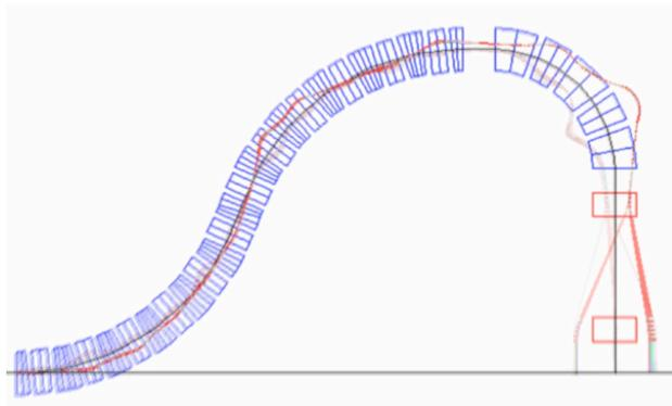
Figure 8: The fixed filed superconducting carbon isocentric gantry with beams of 202, 270, and 400 MeV/u. With the magnified (x10) scanning  $\pm 10$  cm positions.
