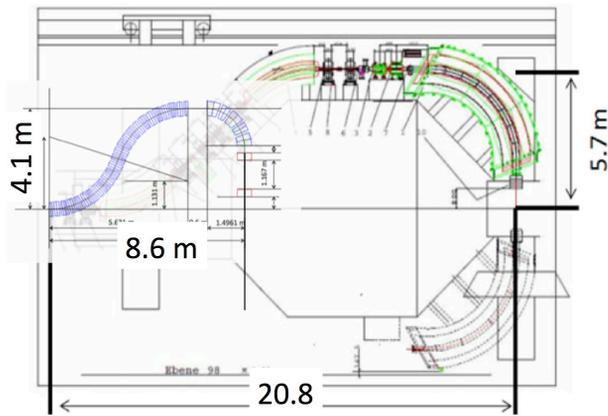
Figure 6: The carbon ion gantry with superconducting magnets is shown together with the Heidelberg gantry.
