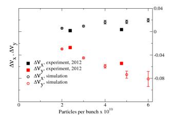
Figure 3: Comparison of the calculated coherent tune shifts for a full machine at injection with measurements. The simulation shows a slightly larger tune shift.
