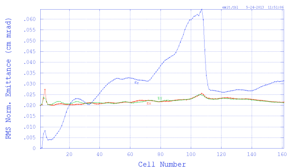
Figure 2: Transverse (red, green) and longitudinal (blue) rms, norm. beam emittances along the RFQ for the design input beam.
