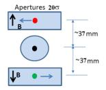
Figure 5: Schematic of 3-way Lambertson magnet. The beam is steered toward the left or the right depending on the sign of the vertical deflection imparted by the VDU.
