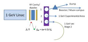
Figure 4: Conceptual design of 1 GeV extraction line.
