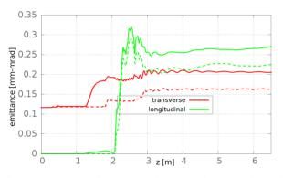
Figure 3: Normalized RMS beam emittances through LEBT and RFQ. Solid: LEBT with un-neutralized section. Dashed: fully neutralized LEBT.
