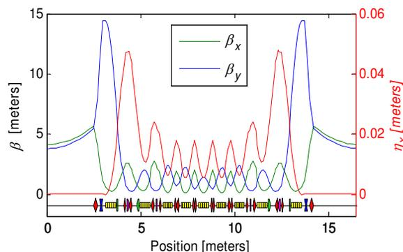
Figure 1: ALS-II candidate lattice Twiss functions.
