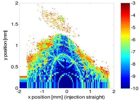
Figure 3: ALS-II lattice dynamic aperture with errors.
