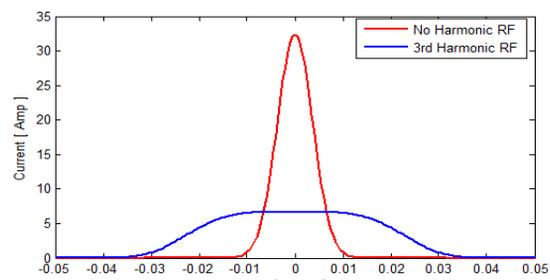
Figure 5: The bunch length of the standard and double RF system.
