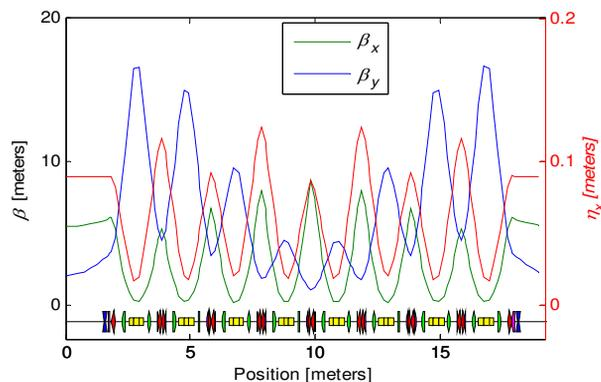
Figure 6: ALS Booster-size Accumulator ring lattice functions.
