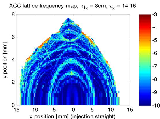
Figure 7: Accumulator ring dynamic aperture.
