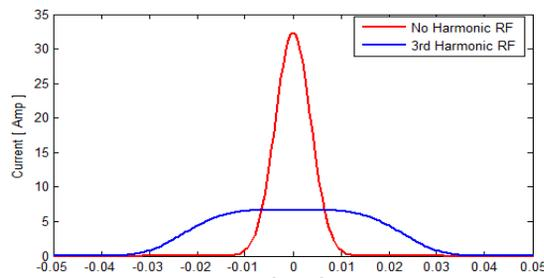
Figure 5: The bunch length of the standard and double RF system.
