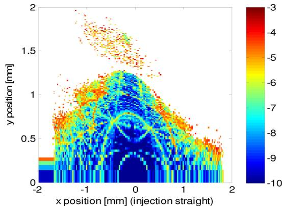
Figure 3: ALS-II lattice dynamic aperture with errors.
