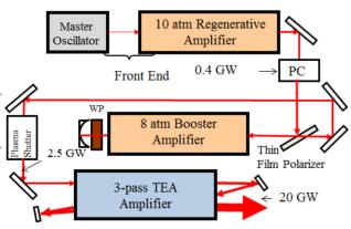
Figure 3: Block diagram of the Neptune Laboratory's high repetition rate system. The orange and blue blocks refer to amplifiers which use pressure and field broadening to sustain ps bandwidth, respectively.
