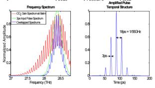
Figure 2: Simulations showing the production of a ps pulse train after amplification of a single ps pulse in a 10 atm CO<sub>2</sub> laser.
