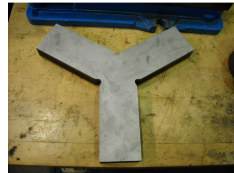
EDM wire cut Nb template for Y WG
