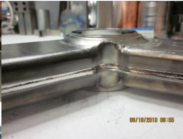
CNC machine two halves and EBW
