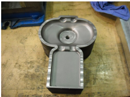
Finished first half with 4mm wall thickness
