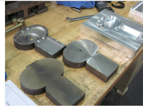
EDM wire cut Nb template
