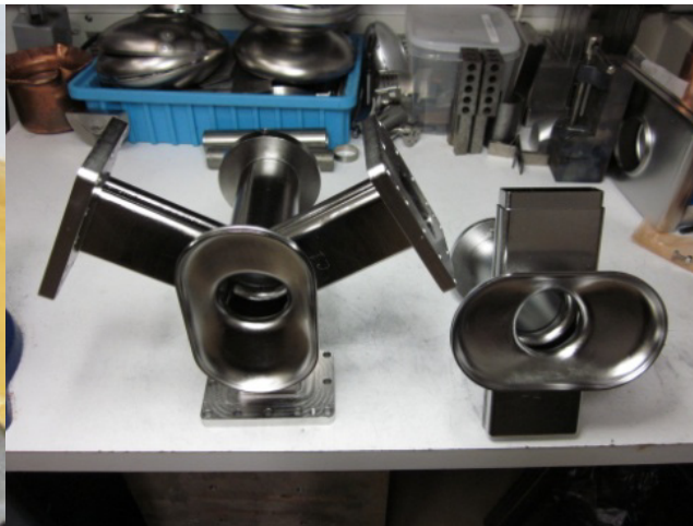
Finished two half groups before final equator EBW
