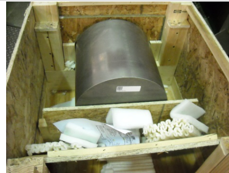
RRR>250 large grain Nb ingot
