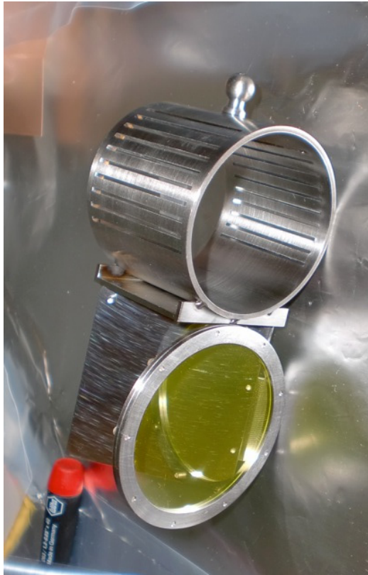
Injector (9MeV) YAG:Ce viewer - for injector phasing, emittance, Twiss parameters, \delta E
