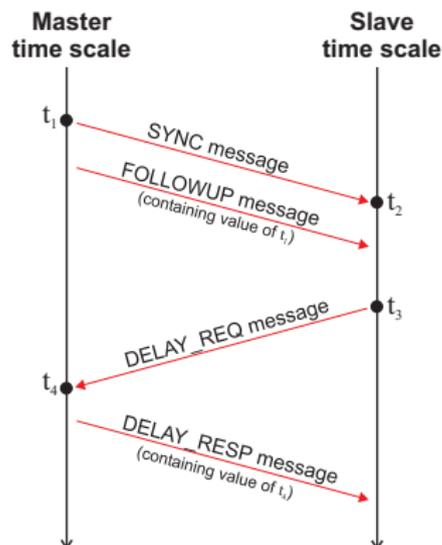
Having the values of  $t_1$ ,  $t_2$ ,  $t_3$  and  $t_4$ , the slave can calculate the one-way link delay:
