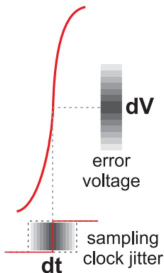
Clock jitter becomes amplitude noise in the sampled signal, with a conversion factor depending on signal slope.
